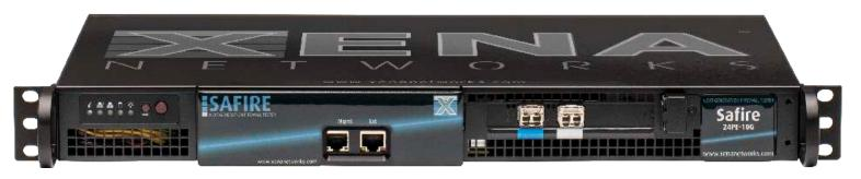
Safire makes it easy to accurately measure the performance of enterprise firewalls. Using traffic that can match the unique traffic profile in your network, Safire pinpoints performance bottlenecks in simple-to-understand graphs, clearly revealing how features like antivirus, appcontrol, IPS and SSL decryption impact throughput.
