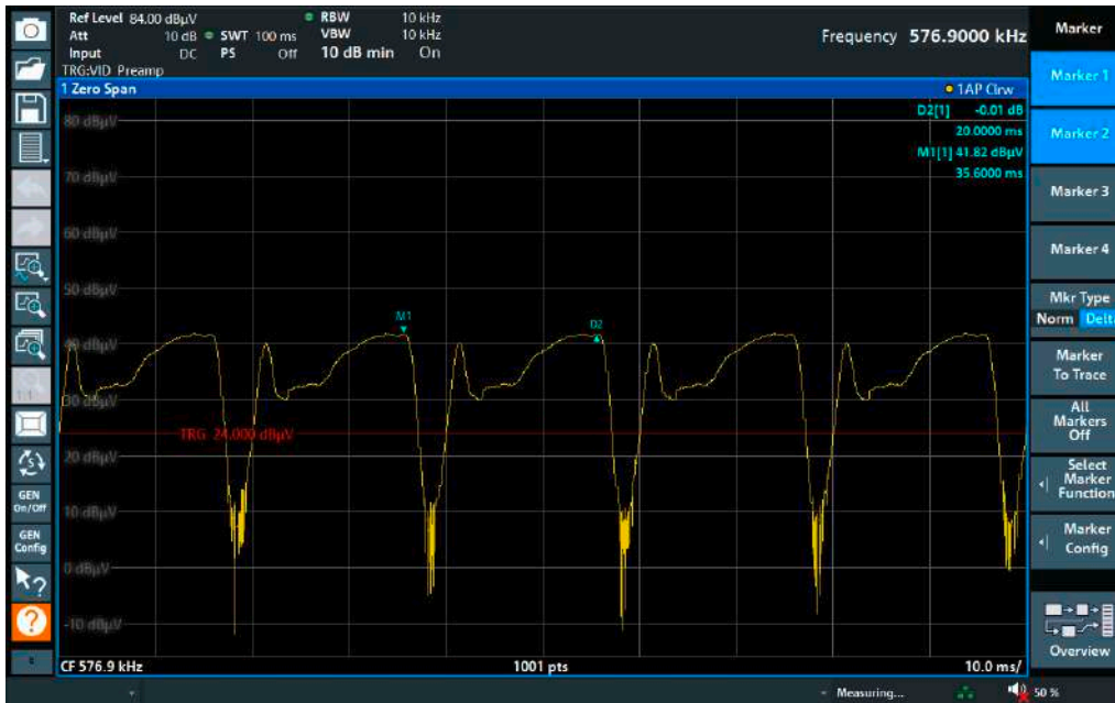
Analysis of the emissions of a LED lamp at 576 kHz versus time. The trigger function ensures a stable display. A period of 20 ms was measured using the marker functions.
