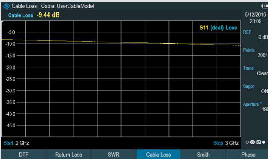
One-port cable loss measurement
