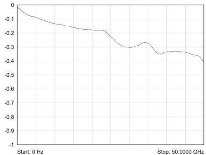
Typical Insertion Loss (dB) Plot for 50 GHz Terminated & Underterminated Versions
