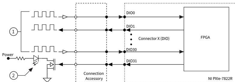
1. High-speed signal frequencies up to 80 MHz with logic levels configured as 1.2 V, 1.5 V, 1.8 V, 2.5 V, or 3.3 V
