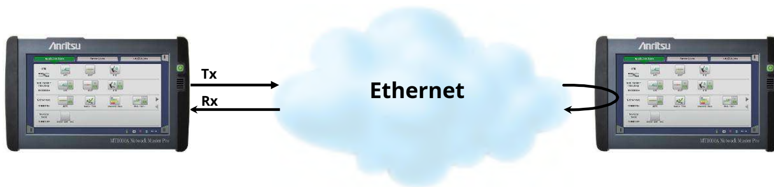
Ethernet testing with far-end reflector
