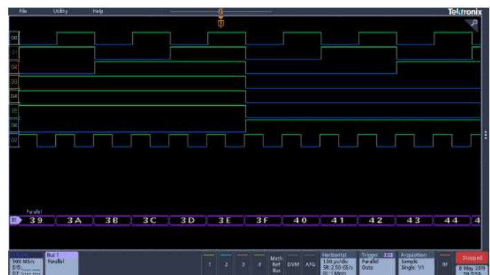
With color-coded digital waveform display, groups are created by simply placing digital channels together on the screen, allowing digital channels to be moved as a group.
