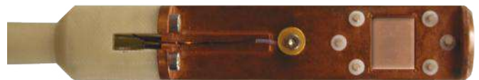
The CCR single sample insert has a sapphire pad and solder posts
