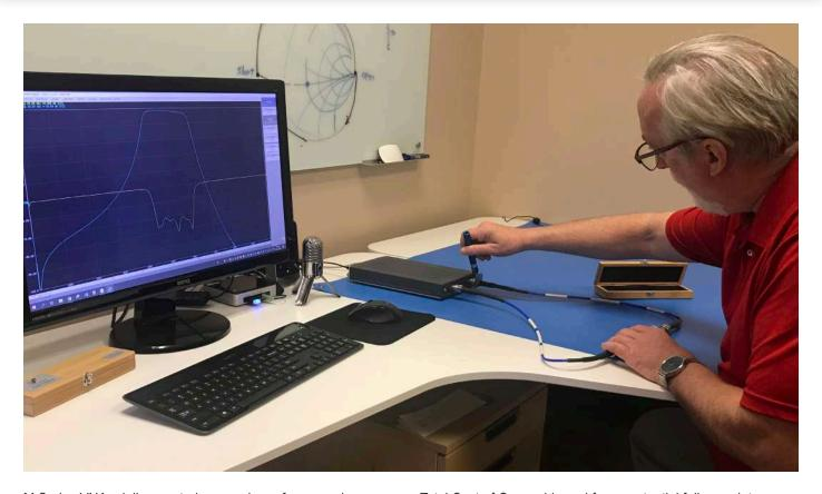
M Series VNAs deliver metrology-grade performance in a more economical package that excludes a number of advanced features: Vector Mixer Calibration, TRL Calibration, Frequency Offset, Time Domain, and Gating. These Vector Network Analyzers are small, can be powered by battery, and are ideal for use in laboratory and production testing in a variety of applications including filter tuning, antenna test and characterization, amplifier testing, etc.
