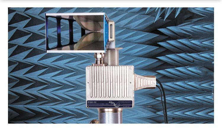
Our 1-Port VNAs (cable and antenna analyzers) perform lab quality measurements connecting directly to the DUT without the need for a test cable, resulting in increased accuracy and quality of VNA measurements, specifically in cable and antenna analysis. In 2016 we were granted a US patent for Measurement Module of Virtual Vector Network Analyzer number US 9,291,657 for this innovation.
