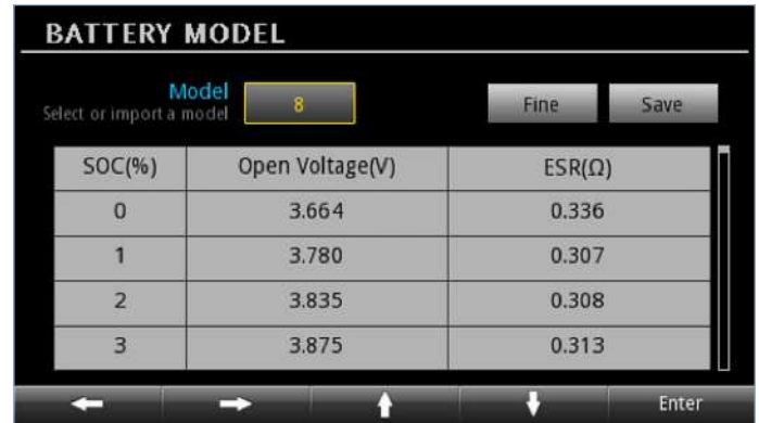
Figure 2. Open a battery model in the 2281S battery test mode.
