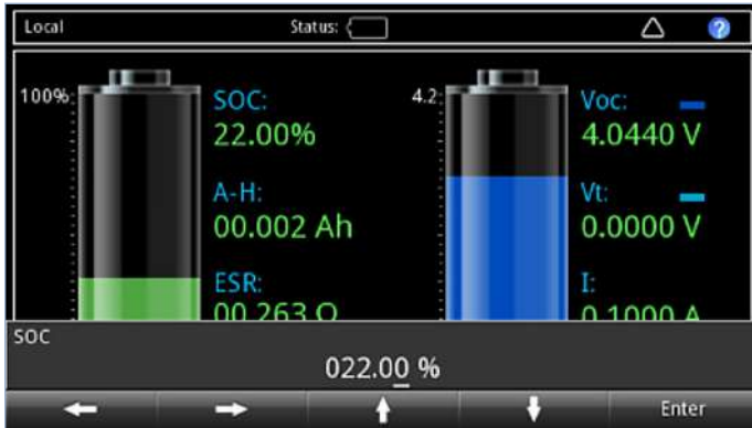
Figure 4. Initiate battery condition in battery simulation mode.
