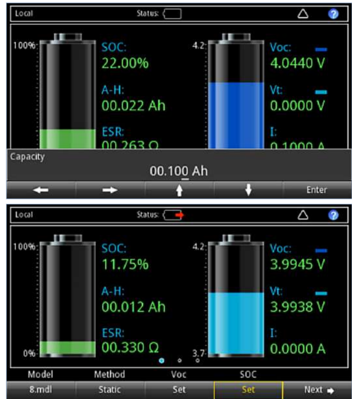
Figure 5. Modify battery capacity to accelerate charge/discharge tests.
