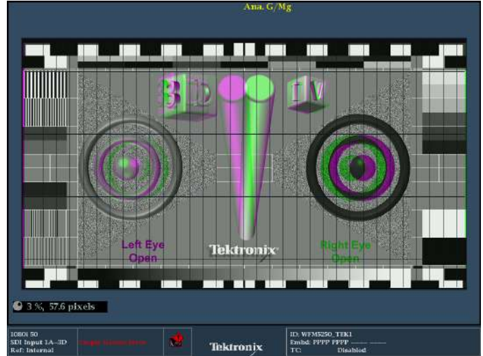
3D monitoring using a disparity grid.
