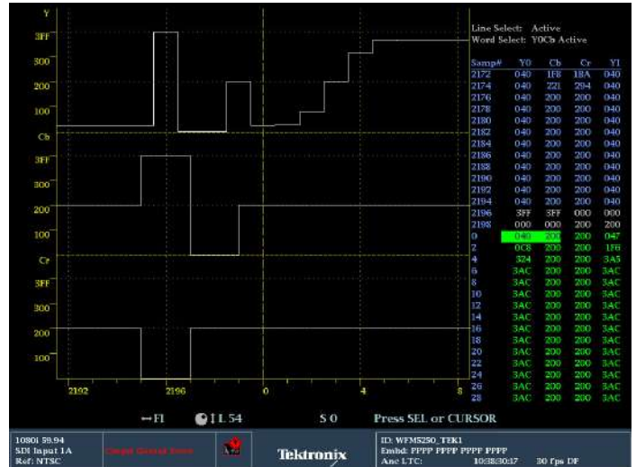
Datalist display provides detailed pixel-by-pixel information.
