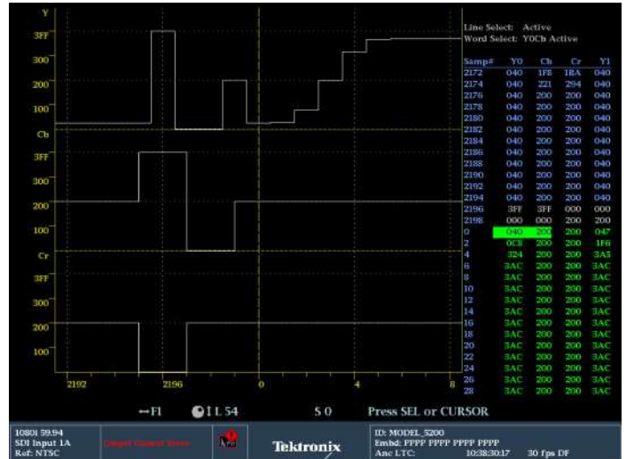
Datalist display provides detailed pixel-by-pixel information.
