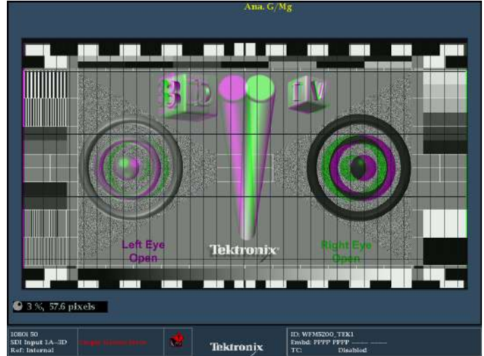
3D monitoring using a disparity grid.
