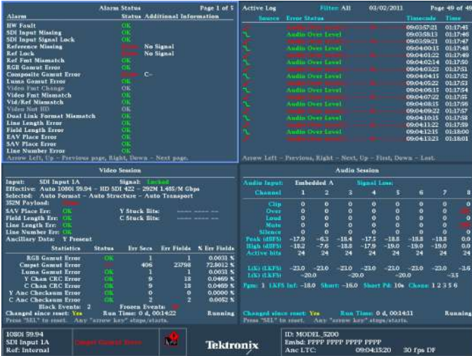
Quad Tile display of Alarm Status, Error Log, Video, and Audio Sessions.
