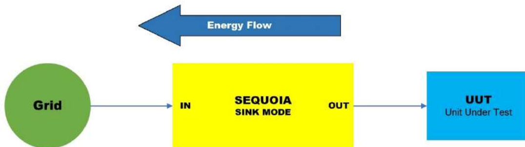
Figure 2-2: Energy flow in SINK operating type
