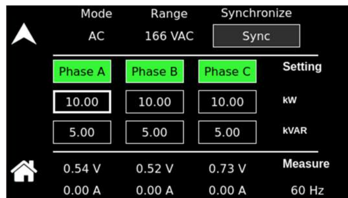
Figure 5-169. Real-Time, Immediate Output Parameter Adjustment
