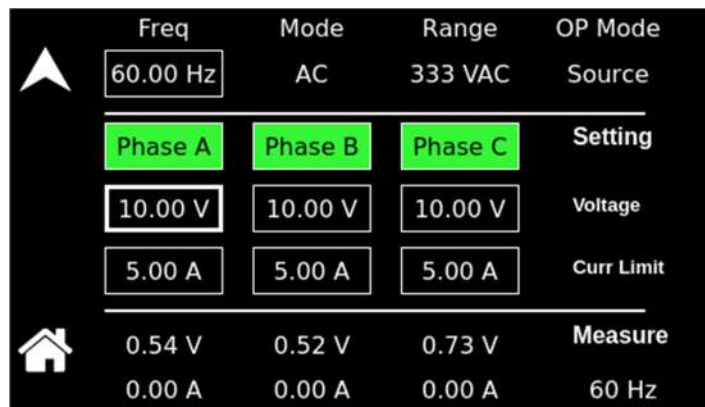
Figure 5-21. Real-Time, Immediate Output Parameter Adjustment
