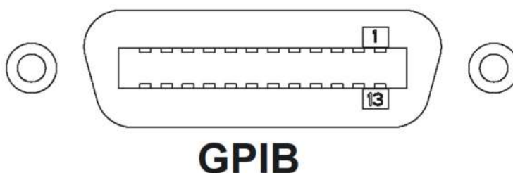
Figure 3-23: GPIB interface Connector
