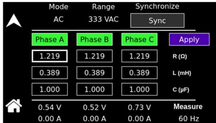
Figure 5-197. Apply button enabled when there is a configuration change
