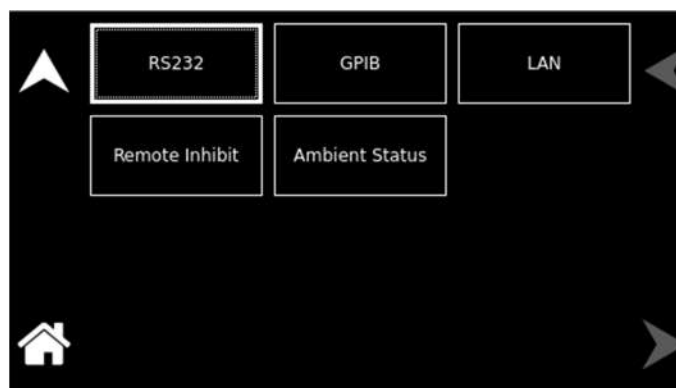
Figure 5-239. CONTROL INTERFACE Screen for eLoad-Power and Parallel RLC Programming Mode
