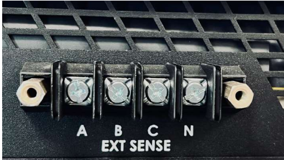
Figure 3-8: External sense Connector
