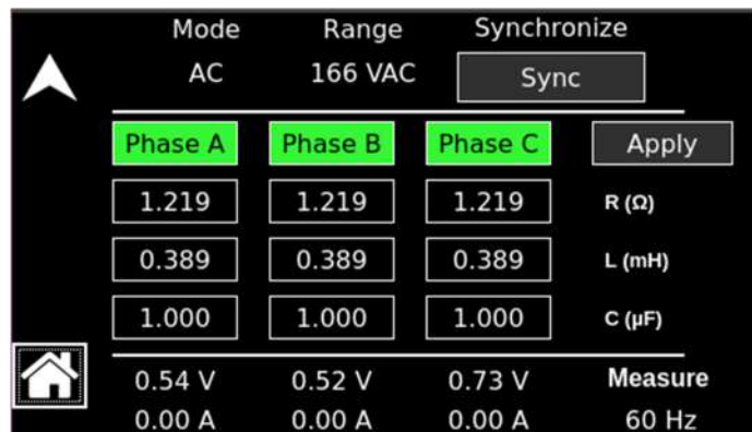
Figure 5-198. Apply button Disabled when there is no change in R, L, or C
