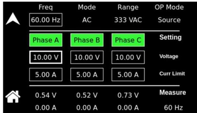
Figure 5-4. DASHBOARD Screen Menu with Voltage Selection-Field Active
