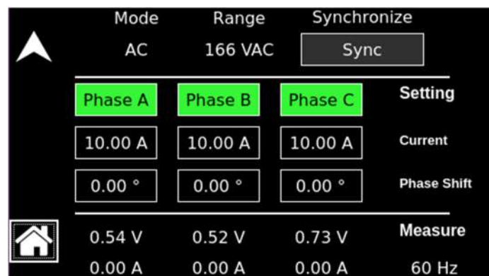
Figure 5-125. Real-Time, Immediate Output Parameter Adjustment
