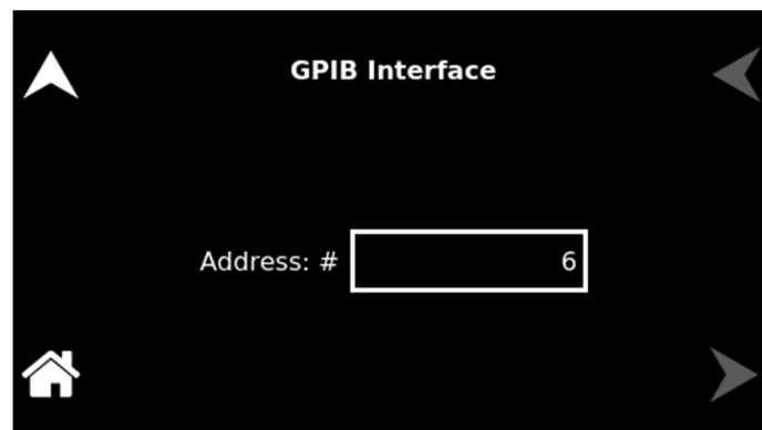
Figure 5-243. CONTROL INTERFACE Menu, GPIB Sub-Menu
