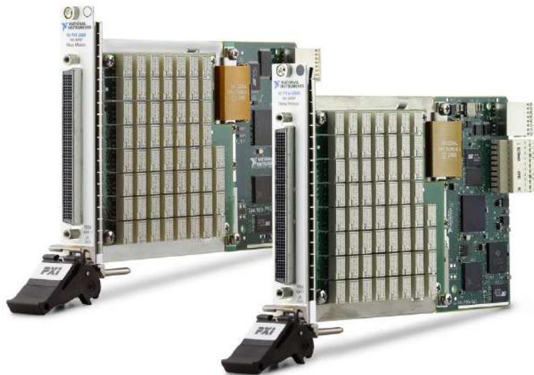
Figure 4. The PXI/PXIe-2569 is one example of a PXI Relay Module that can be reconfigured into either 100 SPST relays or 50 DPST relays.
