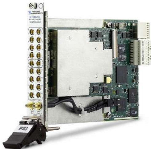
Figure 5. The PXIe-2593 is one example of a PXI RF Multiplexer Switch Module that can be reconfigured into various multiplexer topologies, ranging from a 16-channel, unterminated RF multiplexer to a 2-bank, 4-channel, terminated RF multiplexer.
