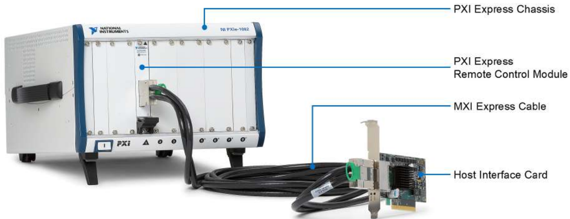
Figure 1. PXIe-8381 (remote control module) and PCIe-8381 (host interface card) allow desktop PC control of a PXI Express chassis with PCI Express Gen 2 x8 data throughput.
