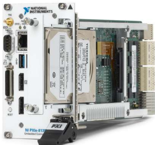
Figure 3: The PXIe-8135 offers a removable hard disk drive.
