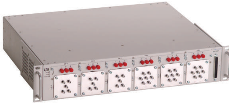
EX72SF with 6 multi-throw and 6 SPDT 26.5 GHz relays
