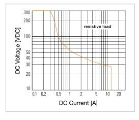
The switching capacity curve shows the maximum voltage and maximum current that can be switched simultaneously by the card. Switching above these limits can reduce life of the relays on the card and is not recommended.
