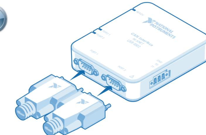
Connect from the DB9 connectors to the CAN bus through shielded cables as described in the *NI-XNET Hardware and Software Help*.
