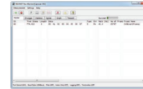
In Measurement & Automation Explorer (MAX), right-click the CAN interface under the device and select Bus Monitor. After selecting network parameters, click the start button to verify functionality.
