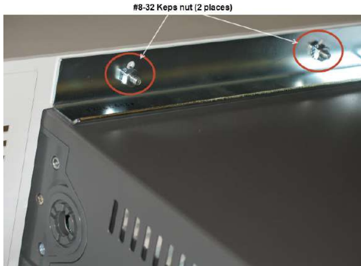
Figure 15: Secure the instrument to the chassis
