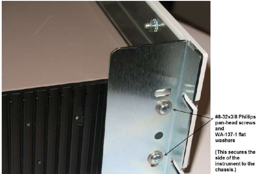
Figure 12: Install the support bracket
