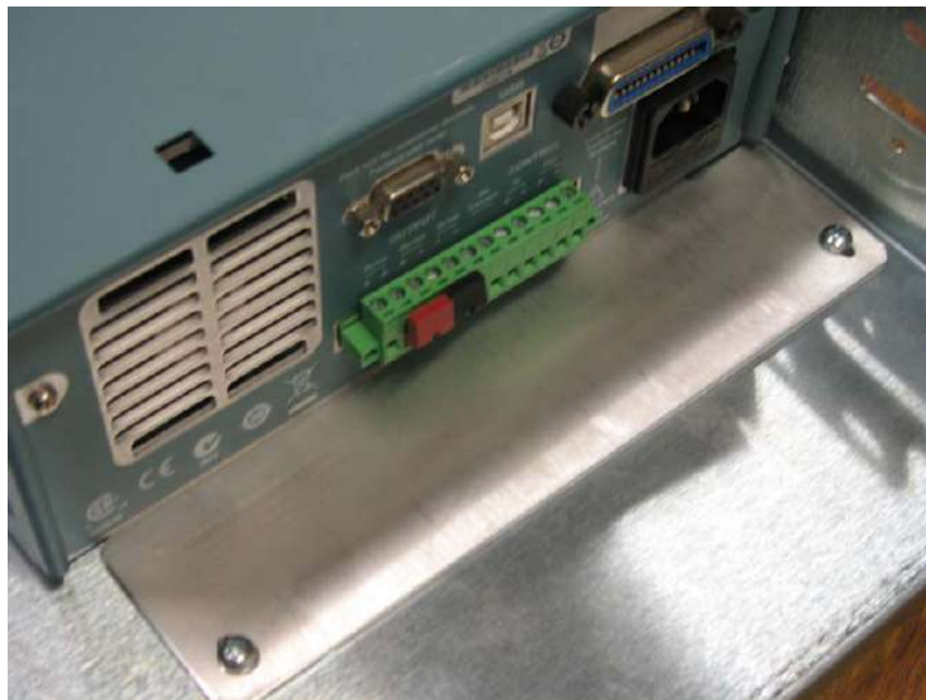
Figure 19: Secure the instrument with the rear clamp
