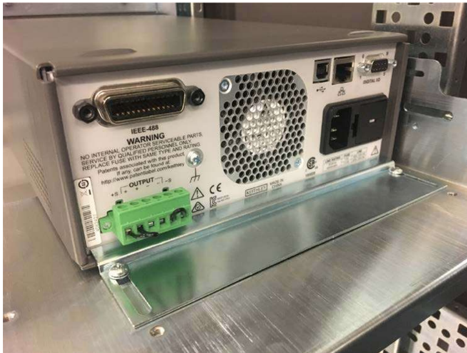
Figure 23: Install the rear clamp
