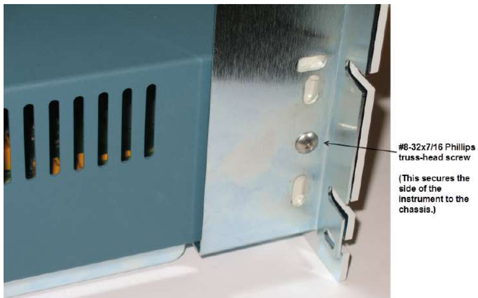
Figure 27: Install the support bracket
