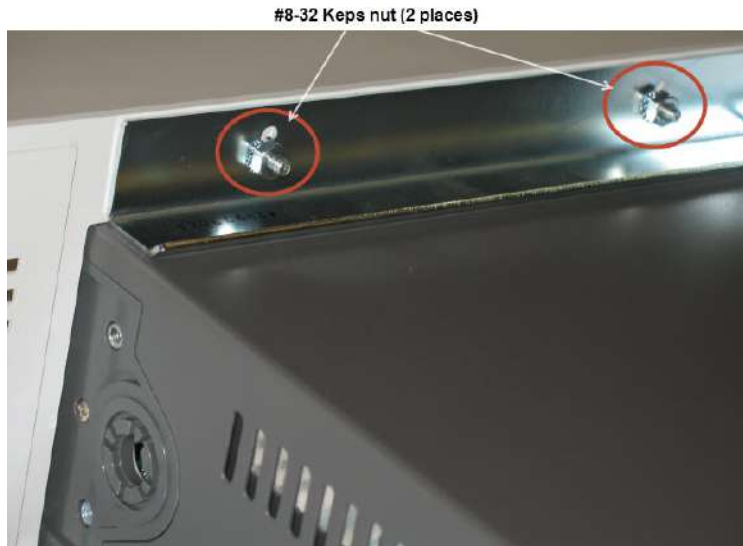
Figure 18: Secure the instrument to the chassis
