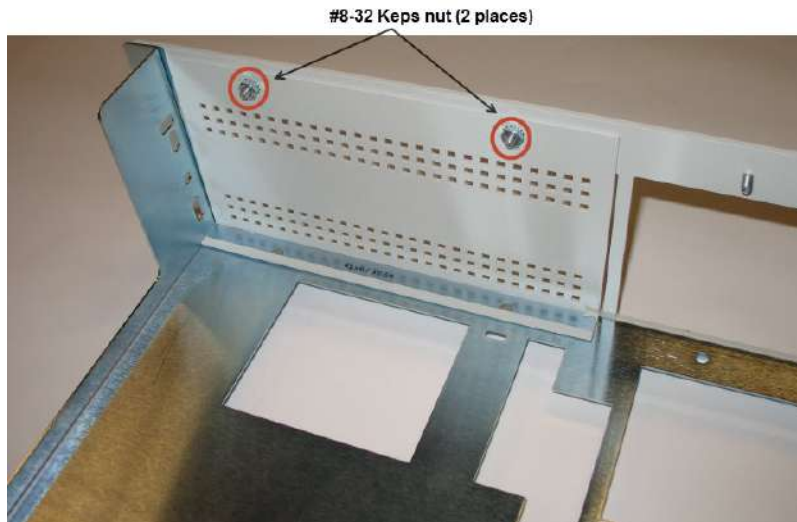
Figure 10: The front-panel plate installed
