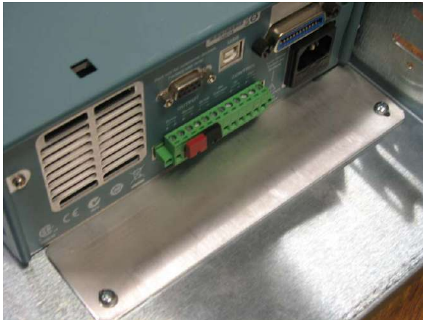
Figure 16: Secure the instrument with the rear clamp
