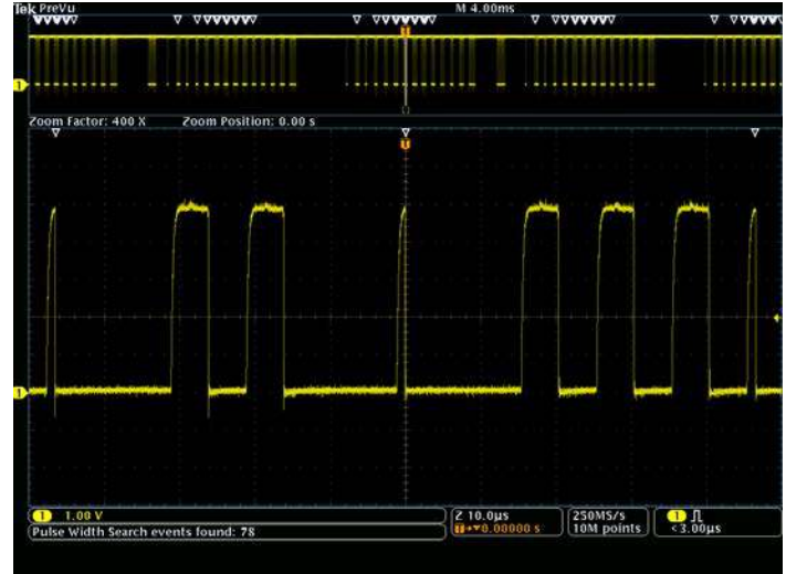
Search step 2: Wave Inspector automatically searches through the record and marks each event with a hollow white triangle. You can then use the Previous and Next buttons to jump from one event to the next.
