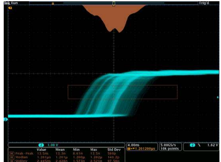
Waveform histogram of a rising edge showing the distribution of edge position (jitter) over time. Included are numeric measurements made on the waveform histogram data.
