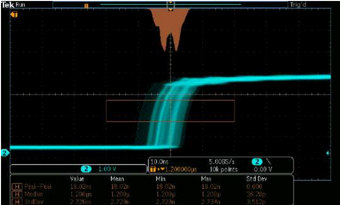
Waveform histogram of a rising edge showing the distribution of edge position (jitter) over time. Included are numeric measurements made on the waveform histogram data.
