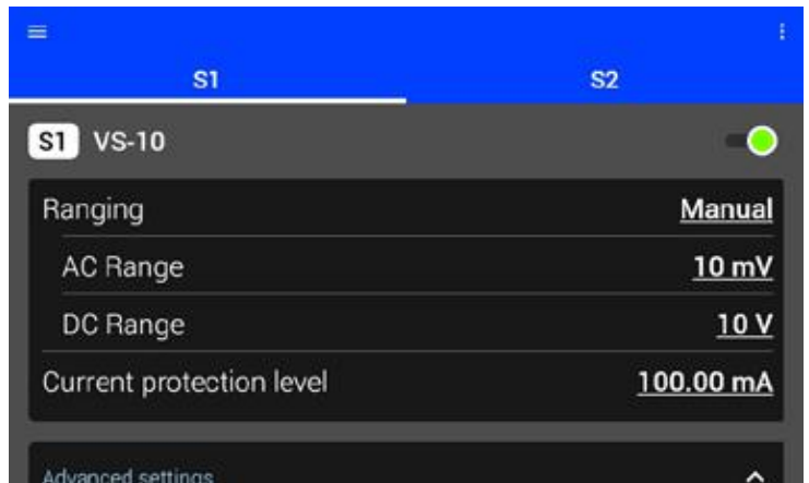
Dual AC and DC range source settings on the VS-10 module enable better control of DC and AC amplitude signals.
