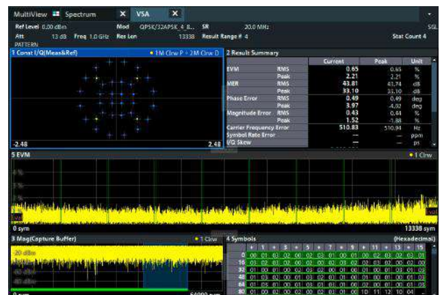
Demodulation of a DVB-S2X multi-modulation signal with the R&S®FPL1-K70M option (R&S®FPL1-K70 option required)
