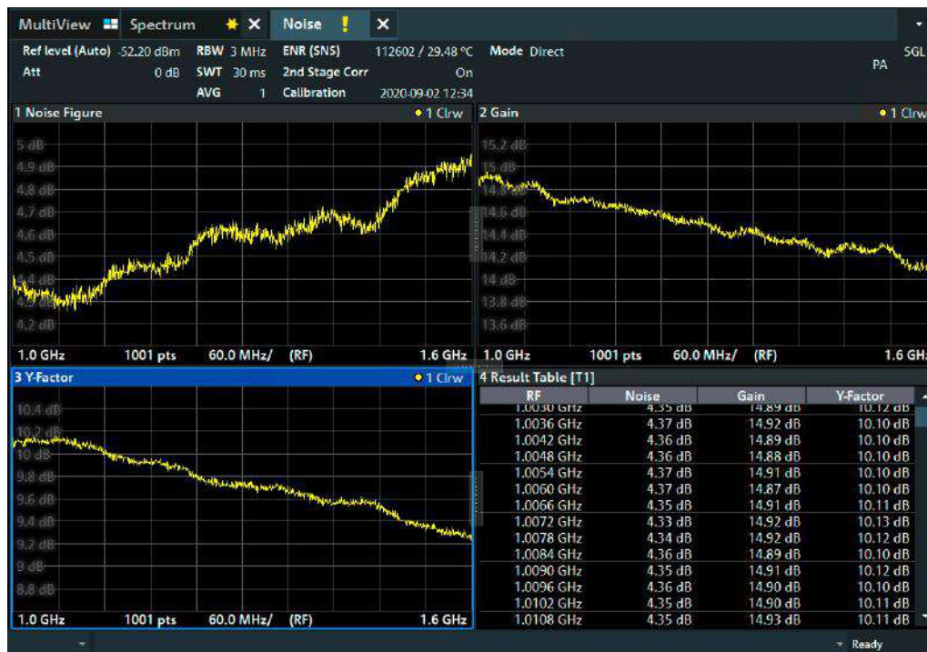
Simultaneous view of graphs for noise figure, gain and Y-factor versus frequency and a table of the results in numerical format
