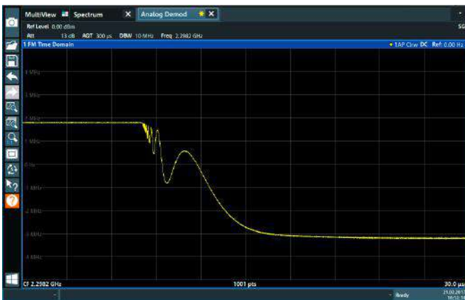
Frequency settling behavior of an oscillator
