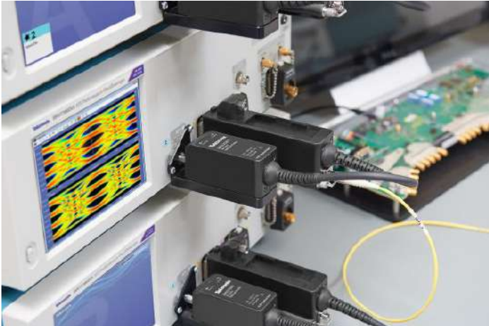
Optical Reference Receiver with controlled response up to 59 GHz on a DPO70000SX oscilloscope's ATI channel
